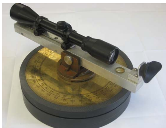
Figure 56 Simple mechanical theodolite
